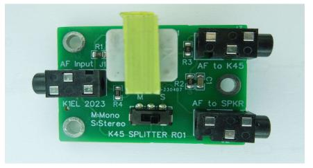
Figure 1 – K45 Audio Splitter board
